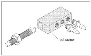
Signal is maintained while stop screw is depressed. Fits all SS stop screws. Operating pressure P=15-120 psi.
