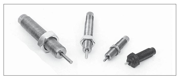
The progressive damping characteristics and built in "self compensation" design, decelerates a moving mass by minimizing the reaction force at impact and gradually increasing the resistance force throughout the working stroke of the shock absorber. (i.e.: higher speeds with softer stops)
